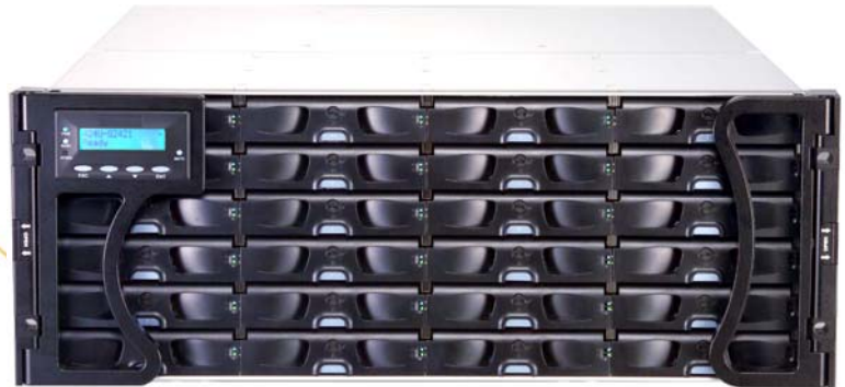
Highest Density today. 18TB in 4U! All disks can safely be removed from the front without moving the chassis! Safe to be rack mounted anywhere in the rack cabinet.
